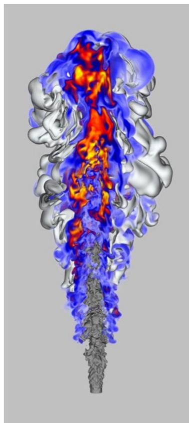
**Figure 9:** This image shows a developing jet diffusion flame simulation run at NERSC using Berkeley Lab’s PeleM code developed as part of the ECP’s combustion application project and with adaptive mesh refinement methods and software from the ECP AMReX Co-Design Center. In fluid dynamics problems more broadly, applied math researchers have used optimization, statistical methods and deep learning to aid in parameter estimation and fast surrogates and to derive highly accurate models from data.
