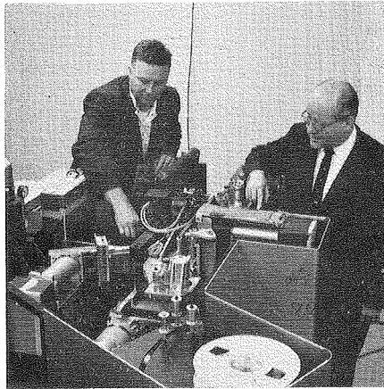
FLYING SPOT DIGITIZER: Above, LRLers Jack Franck (l.) and Howard White demonstrate the Laboratory's first operational FSD model, in Room 2167, Building 50A.
