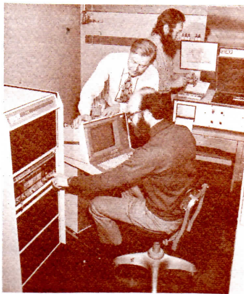
Demonstrating the new computerized lipoprotein scanning system to improve heart disease diagnosis are biophysicist Frank Lindgren (center), research technician Jerry Adamson (rear) and electrical engineer Paul Banchemo. Lipoprotein concentrations in blood plasma samples are measured in the scanning device (background), and the information is fed into the PDP-8 computer.
